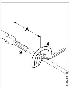
The loop handle can be adjusted to suit the height and reach of the operator and the application by changing distance (A).
