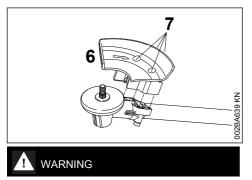
Risk of injury from thrown objects and contact with the cutting attachment. Always fit the limit stop (6) when you use a circular saw blade.
