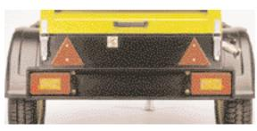
Recessed into the rear chassis rail for protection, the road lighting system comes as standard.
