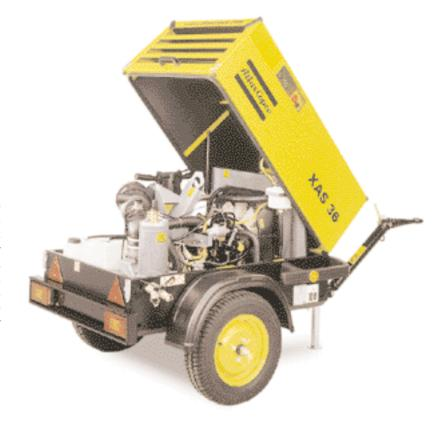
The hood opens wide to give excellent service access and is supported by two gas struts. A new type powder coated zincor steel is used on the bodywork for excellent corrosion resistance. This improves longevity to help the compressor retain a higher residual value.
