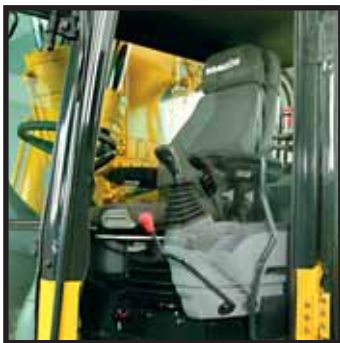
Seat sliding range: 340 mm
