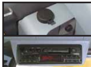
12-Volt power supply and (optional) radio cassette
