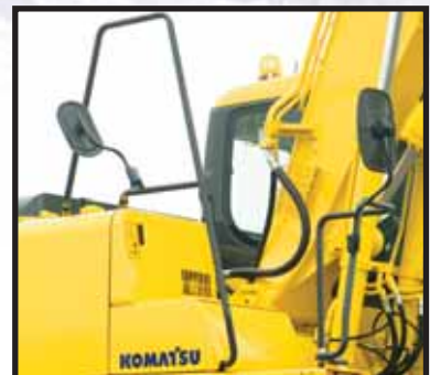
Large handrail for safe access
