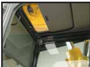
Large sun roof with integrated sun shade
