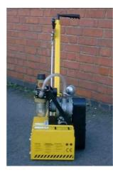
This machine is fitted with the Gast 8AM-FRV-2B Pneumatic Motor with Norgren Oil Fog Lubricator and Controls.
