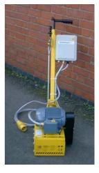
This machine is fitted with the AEG Electric Motor with Moeller Switch Gear, This configuration gives a soft start preventing the normal huge voltage surge caused when the unit is started. The control box has an easily accessible panic stop button and two metre trailing cable with 32 amp plug.
